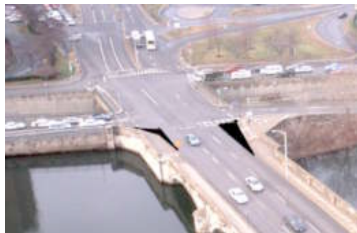
The rounded corners of the River Street make the crosswalk 12ft longer than necessary. By extending the sidewalks 8ft and 4ft respectively, the pedestrian interval cross time could be decreased by three seconds. The black sections show where these extensions should be.
