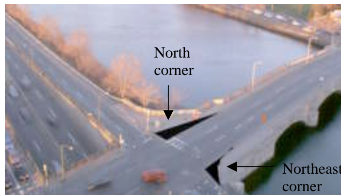
The rounded corners of the River Street make the crosswalk 12ft longer than necessary. By extending the sidewalks 8ft and 4ft respectively, the pedestrian interval cross time could be decreased by three seconds. The black sections show where these extensions should be.
